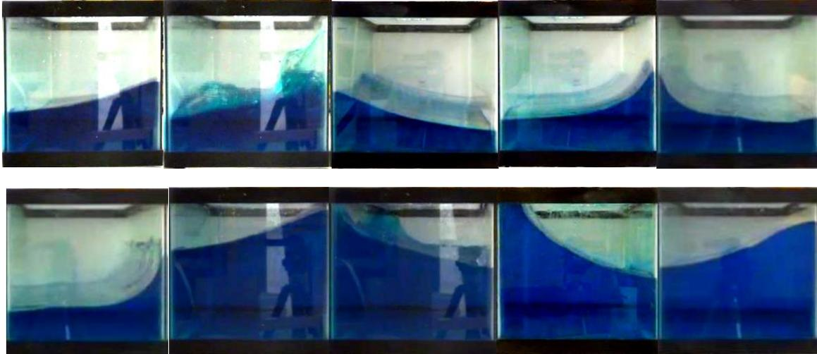
Figure 4- Higher liquid height observed near the corners of the tank in different orientations and excitation types
